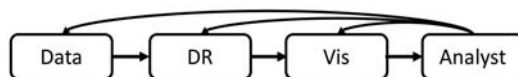
Fig. 1: A basic DR pipeline maps data to a DR algorithm. The results are visualized and presented to the analyst. Interaction feeds back to the pipeline components.
