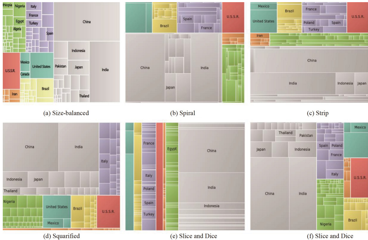
Figure 9 Visual results of the Population dataset. The size-balanced method(a) is compared with Spiral(b), Strip(c), Squarified(d), Slice and Dice(e), and Pivot by middle(f) methods. Leaf nodes with the same parent root share the same color.
