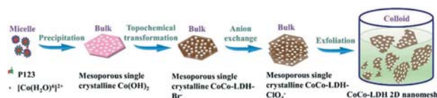
Fig. 21 The schematic of the synthesis process of CoCo-LDH 2D nanomesh. Reproduced with permission from ref. 126.
