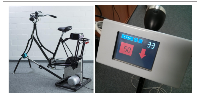
FIGURE 1 | The BrainCycles experimental setup. (Left) Classic Dutch frame and EEG amplifier mounted on the Cyclus2 ergometer. (Right) Handlebar display presenting information about the current and the desired target cadence in rpm.
