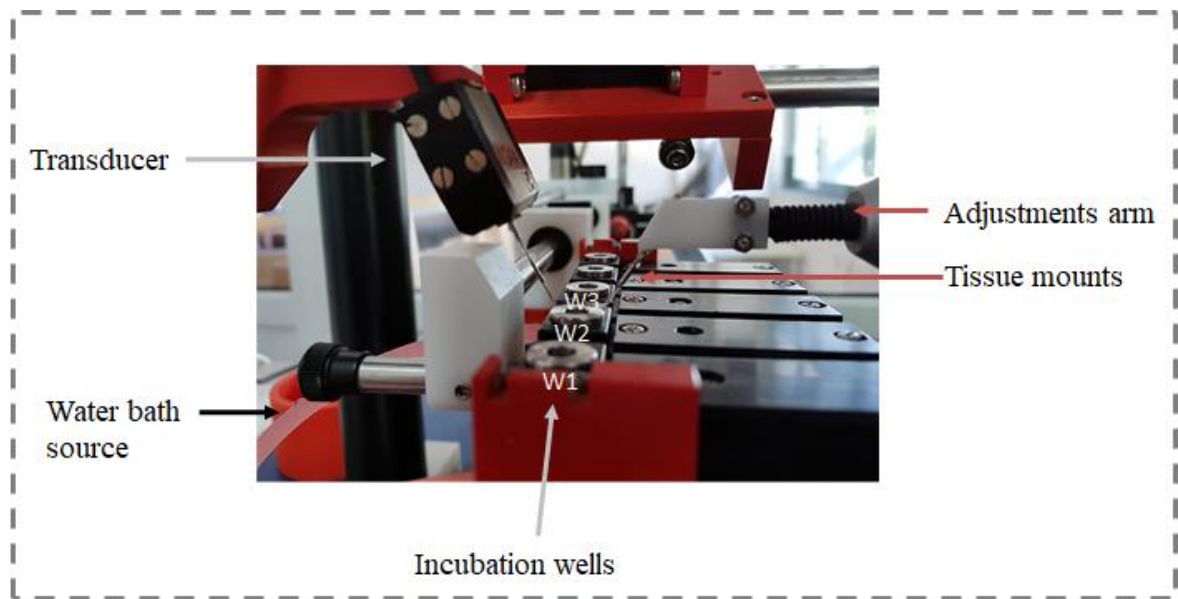
Figure 2.7 SI Heidelberg (WPI) micro dynamometer setup for the muscle fiber isometric tension measurement.
