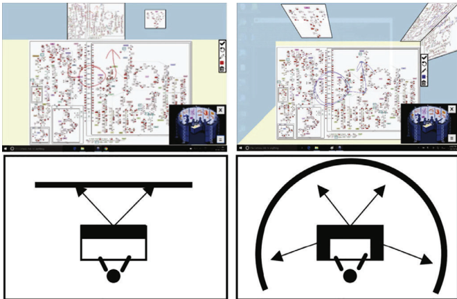
Fig. 7. Two modes of the Windows ContextuWall client can be seen at the top whereas the graphics at the bottom show the application of each mode. The left shows the flat mode used for standard displays and display walls whereas the right shows the immersive mode primarily used for surrounding displays such as the CAVE. The upper screen area shows the interaction area to move, zoom and arrange images on the display. An image can be dragged to the annotation area below the interaction area where graphical annotations can be added. The ContextuWall widget shown in the lower right of each image can be used to drag and drop images from the file manager.
