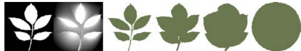
Figure 6: Leaf shape variation encoded in the alpha channel of the texture. From left to right: original leaf texture alpha, radially expanded alpha, shapes obtained with alpha thresholds 0.7, 0.55, 0.4, and 0.25.
