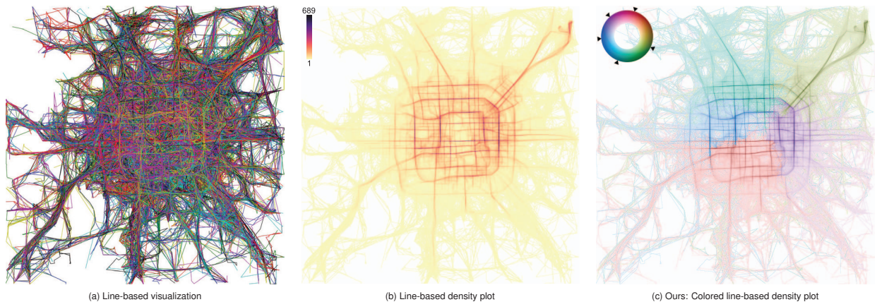
Fig. 1: Trajectories of taxi rides in Beijing: (a) A line-based visualization of the trajectories is cluttered and convoluted; (b) Using a density plot eliminates clutter, but the continuation of the trends is ambiguous, e.g., it looks like taxis follow the prominent, circular route around the city center; (c) Pixel-based colorization reveals clusters, we see that taxis mostly stay in one part of the city.
