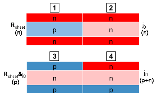
Figure 2: Sample structures for R_{sheet} and j_0 investigation of p^+ emitter and n^+ FSF.
