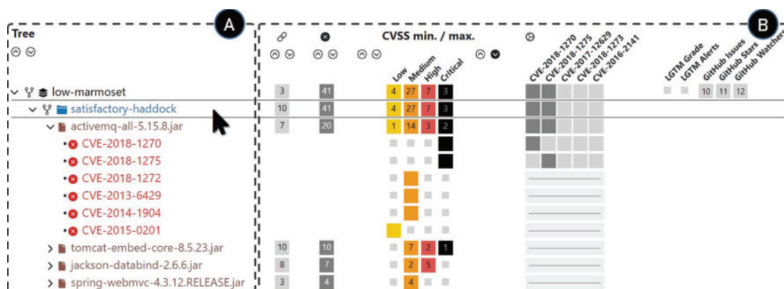
Figure 1: VULNEX is a tool for the investigation of exposure to open-source software vulnerabilities on an organization-wide level. The tool shows repositories, modules, libraries, vulnerabilities in a tree representation (A), and meta-information about each entry (B), such as the CVSS score. We can see that the "low-marmoset" repository is exposed to severe vulnerabilities, three critical and seven high. Two of the critical vulnerabilities are originating from the activemq-all indicating that the library should be updated swiftly.
