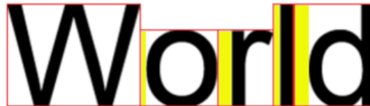
Figure 5: Solution to the constraint solver loop problem: By filling the spaces between the characters no loop can occur.
