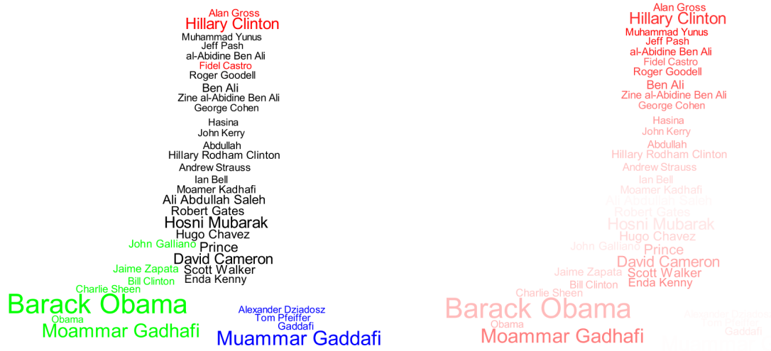
Figure 50: Left: Overlaps removed by Box2D. Right: Amount of displacement of the tags indicated red.
