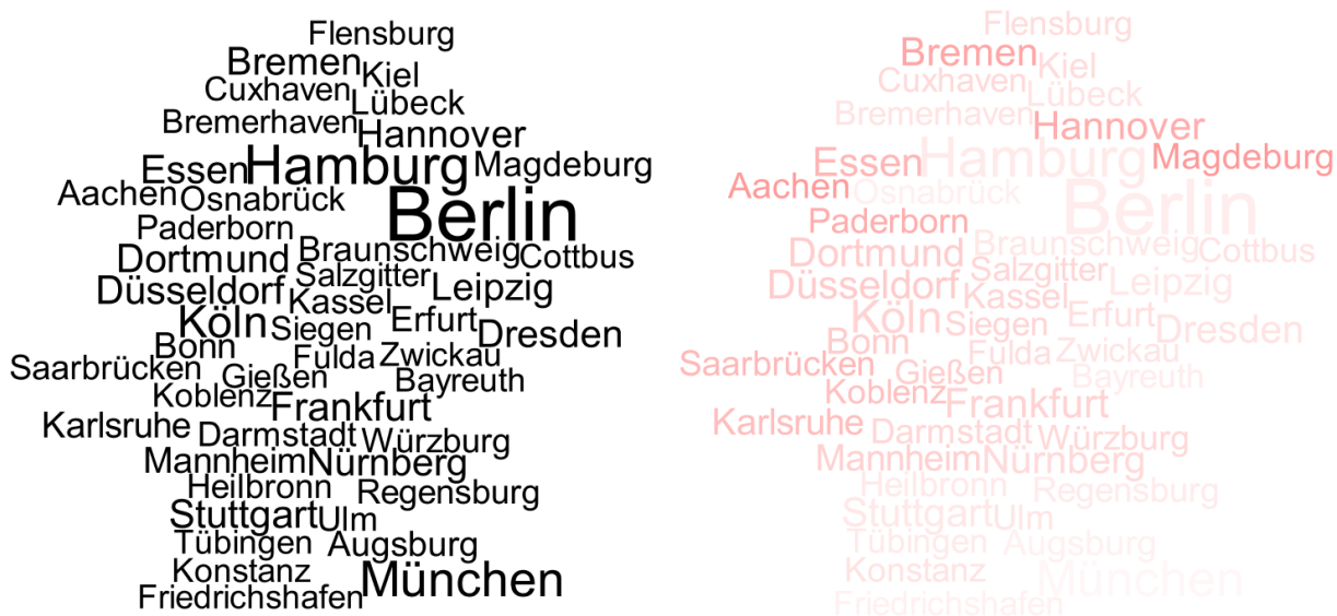
Figure 39: Left: Map of Germany with overlaps removed by Scanline Wordle . The layout is compact and the initial structure is preserved. Right: Amount of displacement (Euclidean distance) of the tags indicated red.
