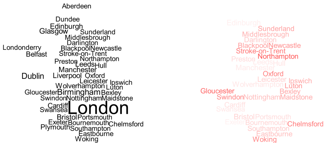
Figure 43: Left: Map of England with overlaps removed by Wordle . The layout is compact, but lacks the structure of the initial layout. Right: Amount of displacement (Euclidean distance) of the tags indicated red.
