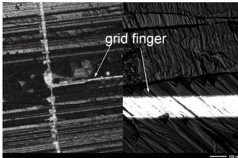
Figure 7.11: Micrograph of a photolithographic (left) and a evaporated (right) front grid on a Recrystallised Wafer Equivalent on RBSiC ceramic substrate.
