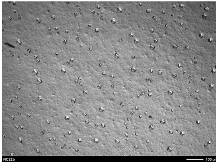
Figure 5.13: Micrograph of a SiC layer as deposited on a silicon substrate with occurring hydrogen blisters.
