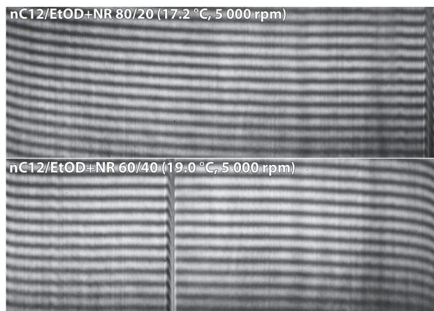
Fig. 12 Experimentally obtained interference fringe pattern corresponding to the fluctuation expected from theory as shown in Fig. 10. Raw images obtained, showing the narrow turbidity zone appearing at 5000 rpm far away from the critical point (top) and close to the critical point (bottom). The discontinuity in the fringe pattern is clearly visible as vertical line similar to a meniscus. Fig. S9 in the ESI† shows an overlay of fringe patterns and composition profiles.
