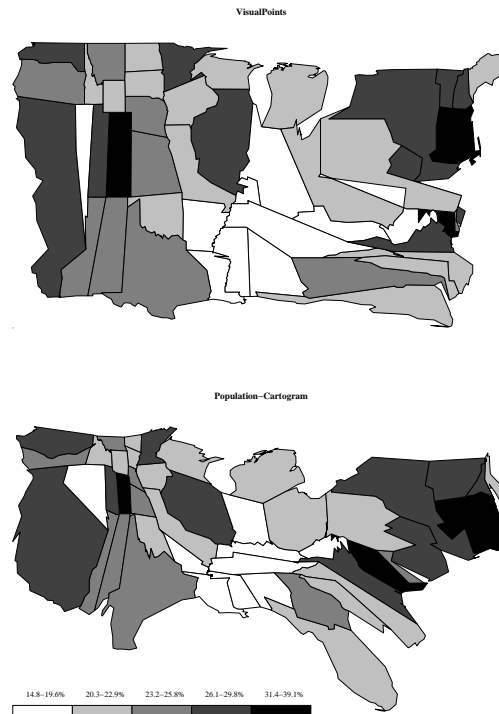
Fig. 6. The Figure displays (1) the U.S. state population cartogram computed with VisualPoints , and (2) the U.S. state population cartogram computed with CartoDraw showing the accomplished bachelor degrees or higher in the USA in 2000. The area of the states in the cartograms corresponds to the population and the grey level of the areas correspond to the percentage of the accomplished bachelor degrees or higher.
