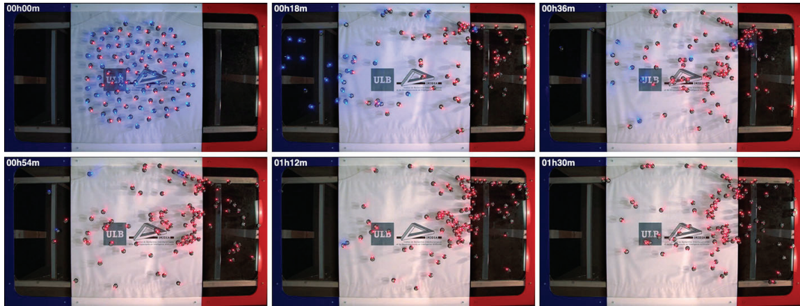
Fig. 4 The figure shows a series of screen-shots taken from one experiment with a swarm of 100 Kilobots. The screen-shots are taken every 18 min of execution (Color figure online)
