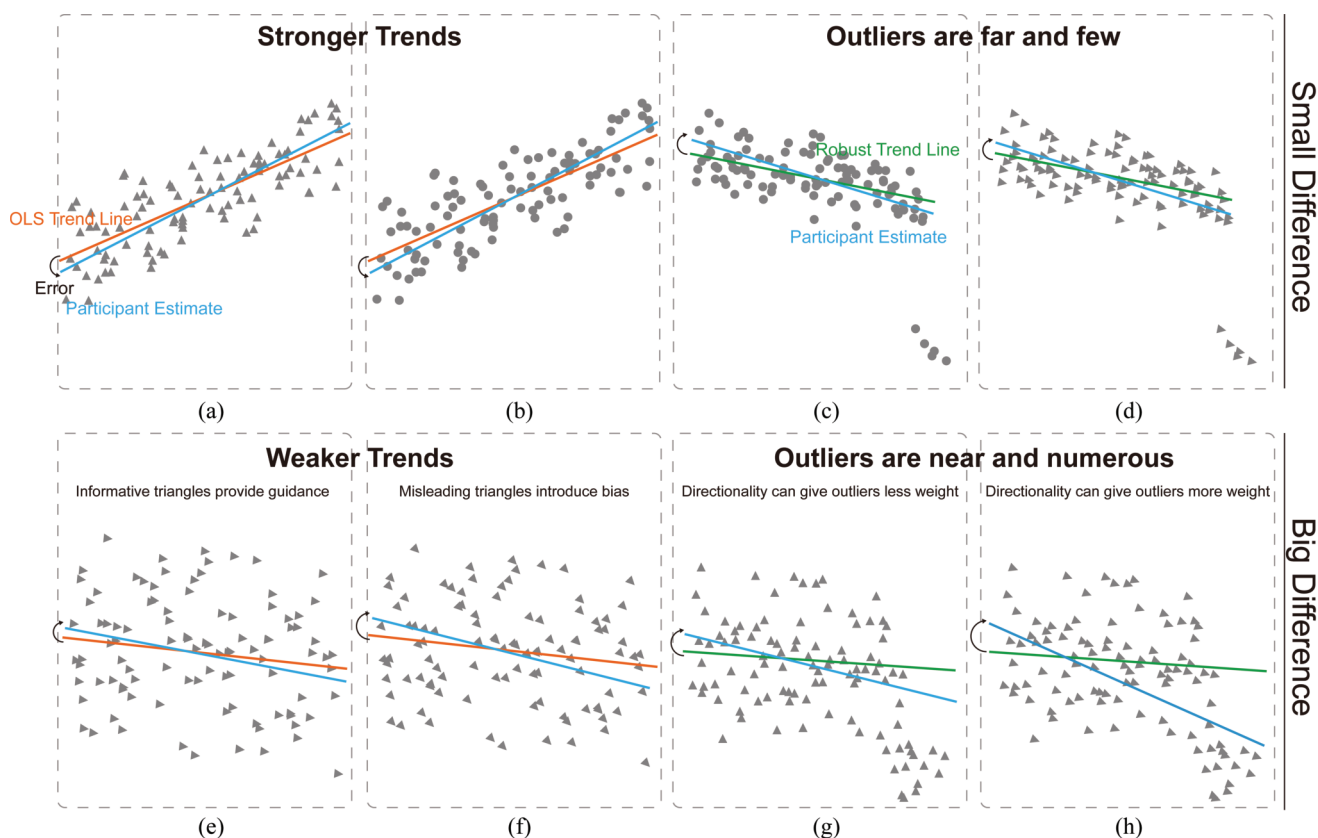
Figure 1: The impact of mark orientation on trend estimation. When a trend in the data is unambiguous, either due to a strong correlation (a,b) or the presence of an obviously outlying cluster irrelevant to the central trend (c,d) mark orientation does not greatly impact the perception of trends in the data. However, when trends are ambiguous, mark orientation can introduce a bias. By using a data-driven orientation of marks in such cases, we can guide viewers to more accurate estimates of weak trends (e,f), or trends impacted by nearby outliers (g,h). This results in estimates that are robust even for cases when assumptions about an underlying linear modeling are violated.
