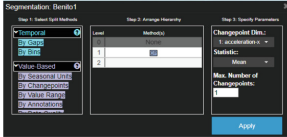
Fig. 4.2 The visual query language interface: In the left column, multiple time series segmentation methods can be selected. The hierarchy of applied methods can be changed via an interactive interface, shown in the second column. Finally, detailed settings for each method can be changed in the third column
