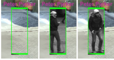
Figure 6. Automatic detections can be displayed as MBRs (left), snippets from video footage (center) or the best-shot of the entity from the entire scene (right).
