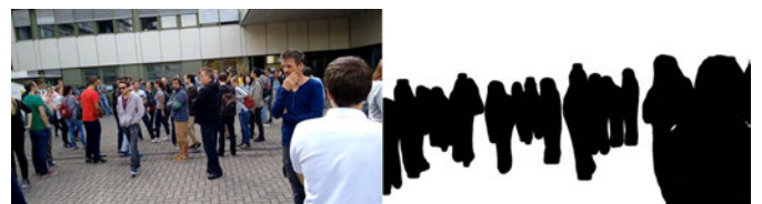
Figure 1. The binary mask to separate static and dynamic scene parts based on Mask R-CNN.
