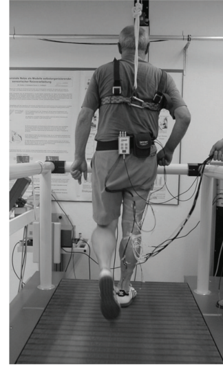
FIGURE 6: Assessment of reactive balance performance using a motorized treadmill (i.e., unexpected decelerating gait perturbations during walking will be applied).
