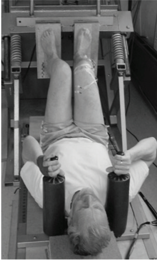
FIGURE 4: Assessment of maximal isometric strength and rate of force development using a leg press (i.e., force signals will be recorded by a separate force plates underneath the feet).
