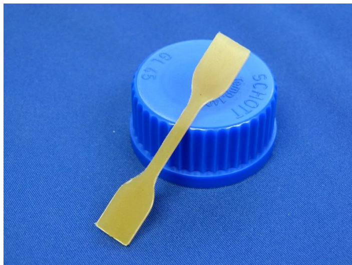
Figure 5.5: Dog-bone-shaped sample bar for tensile testing.
