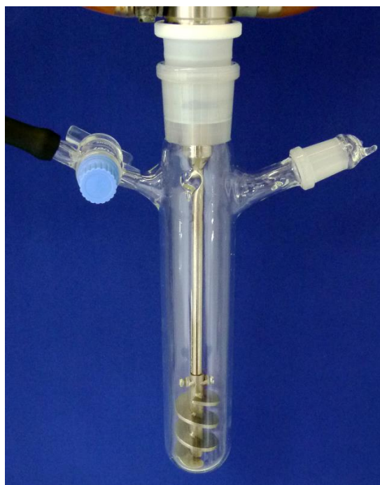
Figure 5.1: Optimized polymerization equipment with a helical stirrer.
