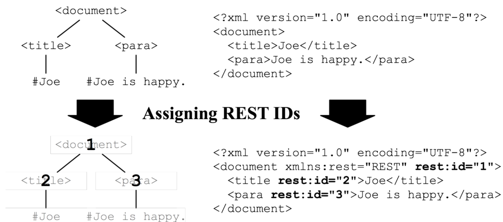
Figure 2. Assignment of REST IDs. Any XML fragment or document can be depicted as an unranked ordered tree. The REST ID makes sure that every element node gets its own unique immutable identifier. ‘<’ and ‘>’ denote element nodes and ‘#’ denotes text nodes in the node tree. A simple XML resource storing a document serves as an example.
