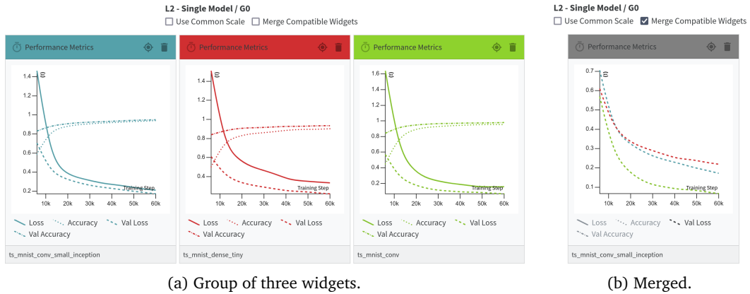
Figure 4.10: iNNspector’s widget group view. (a) Grouped widgets can be opened in a detail view, showing them side-by-side in an enlarged page overlay. (b) Widgets featuring compatible data can be chosen to either use a common scale or be merged into a single meta-widget.
