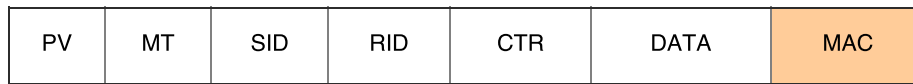
Figure 3.7.: This is the structure of a data message. It consist of protocol version (PV), message type (MT), sender id (SID), receiver id (RID), counter (CTR), payload (DATA) and message authentication code (MAC) of everything before. The payload consist of a reference to a message, a plaintext message (even empty), zero or more TLV records and a signature with the short-lived key of the first 3 items.
