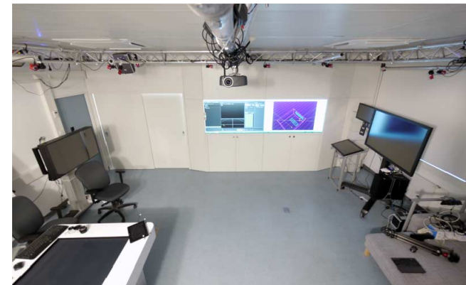
Figure 10. Study lab equipped with 24 optitrack cameras connected to the proximity toolkit [7]. The setting allows for precise tracking and controlled lab studies.
