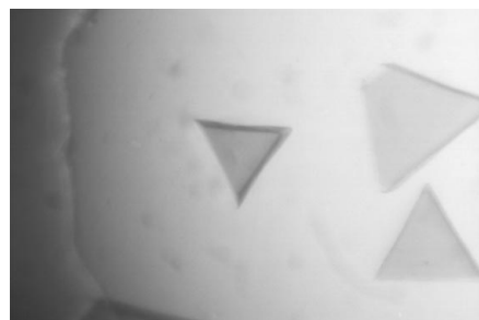
Figure 3 Crystals of transhydroxylase obtained by sitting-drop vapour diffusion in an \text{N}_2/\text{H}_2 atmosphere.
