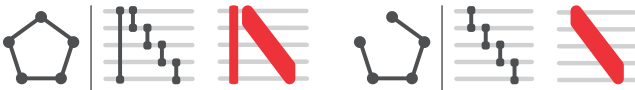
Fig. 12: How to draw a path in BF? Both a closed and open path could be highlighted through bands, ordering first through top node index, then bottom node index.
