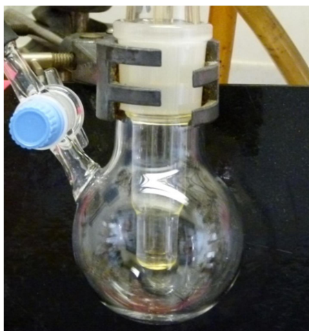
Figure 6.4: Cooling finger used for purification of long-chain aliphatic diisocyanates via distillation.
