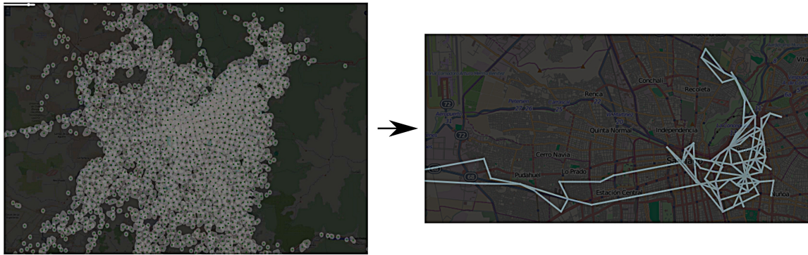
Figure 5.2: Trajectory of a selected user with 500m radius cluster centroids taken as the consecutive user locations.
