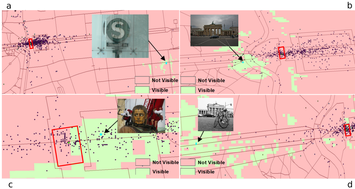
Figure 3.5: Reverse-viewshed from four exemplar observer positions (indicated with the arrow head, and the image taken from the position) to the Brandenburg Gate (indicated with the red rectangle). (a) image is incorrectly geotagged and incorrectly labelled, (b) image is incorrectly geotagged, but correctly labelled, (c) image is correctly geotagged, but incorrectly labelled, and (d) image is correctly geotagged and correctly labelled.
