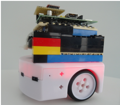
Figure 5: Thymio II robot with a Raspberry Pi and an ambient light sensor attached on top.
