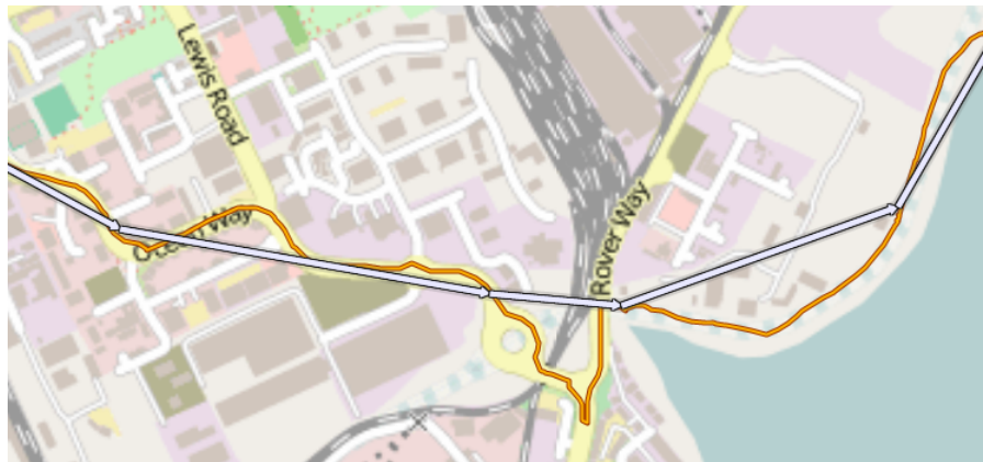
Fig. 7. Comparison between the accuracy of the Garmin GPS sensor ( orange line ) and the ViewRanger app using a smartphone sensor ( white line ). The difference in sampling rate is clearly visible as the ViewRanger only captures the rough direction and the Garmin the exact route.
