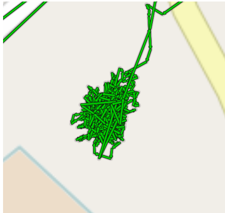
Fig. 10. Image showing a cluster of GPS Track-Points on the rote. There are about 1000 points contained in the cluster and the diameter is about 40 meter.
