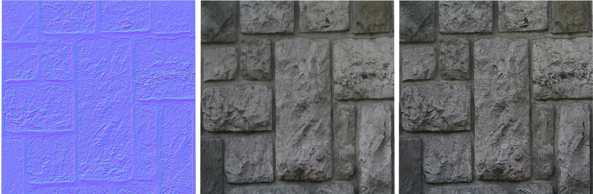
Figure 25: Normal mapping applied to a brick wall texture: the left image shows the normal map for a given brick wall texture. The brick wall texture is rendered without (center) and with (right) normal mapping.
