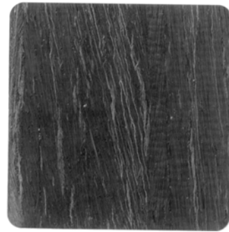
Figure 7: 30 \times 30\ \text{mm}^2 Secco etched sample. The grey level is correlated with the structural defect density. High disorder is visible at the center of this sample.
