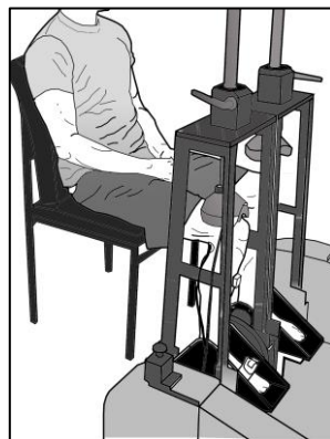
Fig. 2: The participants' right leg was fixed within the ankle dynamometer, which measured the isometric twitch force of the plantar flexors evoked by stimulation of the tibial nerve in the popliteal fossa subsequent to the 4 different types of conditioning and control.
