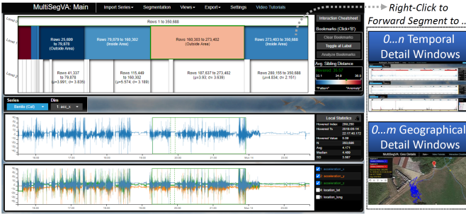
Fig. 3. The main window (with its segment tree visualization and time series plots) that enables to send segments to n + m detail windows.
