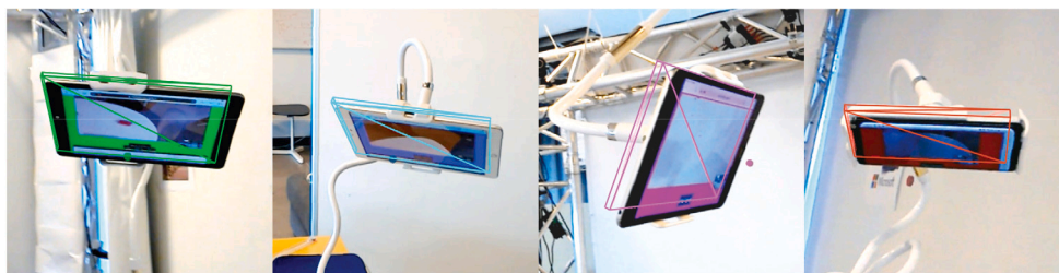
Fig. 5. From the point of view of the worker's Hololens in AR after calibration: The four scene cameras are augmented with the wireframes of their corresponding virtual cameras. In the Virtual Hand + Color Cue condition, the wireframe of each camera has a distinct color, while in the other awareness cue combinations all wireframes are green. (The misalignment of wireframes is a result of the screen capture method. Alignment is accurate, when seen through the HMD).
