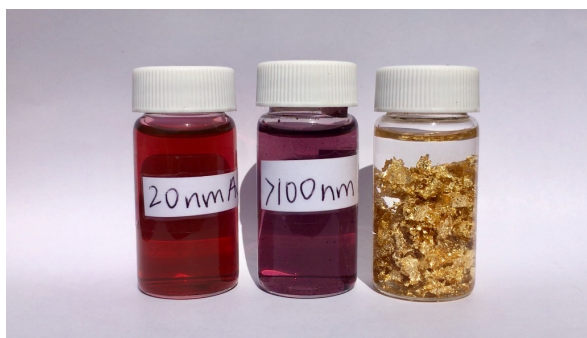
Figure 1.1: Nanoscale gold as an example for the fundamental changes of a materials appearance at different sizes. Adapted from Sustainable-nano.com. 2
