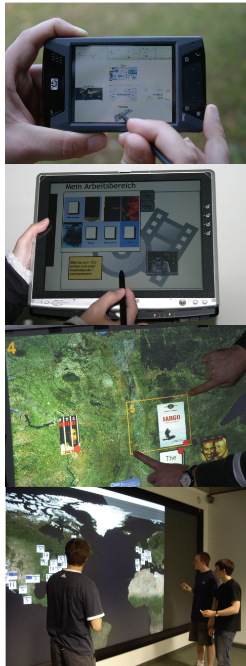
Figure 8. ZOIL-based user interfaces on a PDA, Tablet PC, Multitouch Display and a large high-resolution display.
