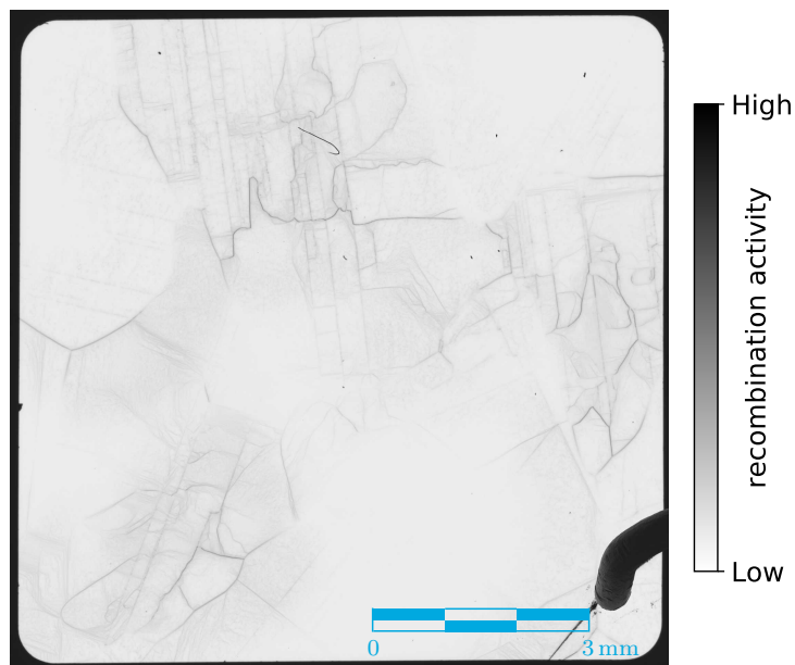
Figure 3.17.: EBIC data of a typical as-grown mc-Si sample. The material shows line-like structures as well as weaker cloud-like regions of enhanced recombination activity. Not all of the line-like structures are originating from grain boundaries [60]. The thick black structure in the lower right corner is the tip of the EBIC current probe that is contacting the aluminum pad.
