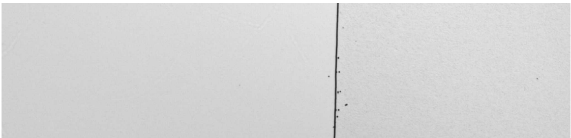
Figure 5.1.: A 1.5 mm wide section of the surface of a gettered wafer after Secco etch (a region of low EPD on the bottom left of same wafer that is depicted in figure 5.10a). Etch pits that are still present after gettering steps tend to be located close to grain boundaries.
