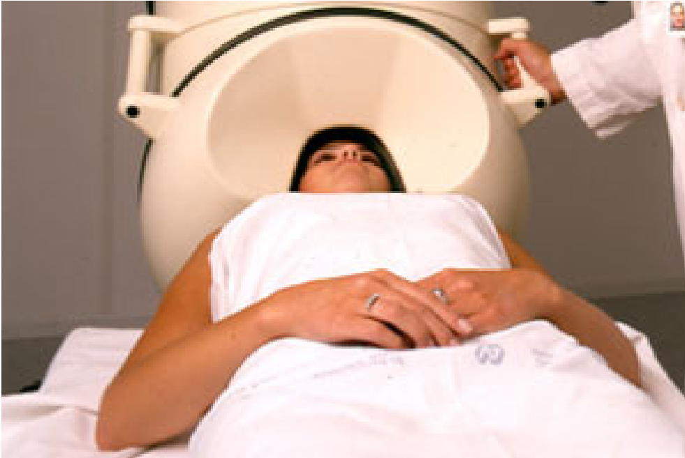
Figure 7: MEG device. The SQUIDs with the pick-up coils are housed in a Dewar that is filled with liquid helium. The Dewar surrounds the scalp in a distance of about 10-15 mm. Experiments can be done in a supine or sitting position.
