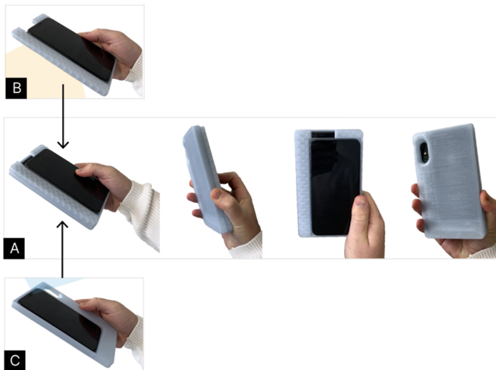
Figure 4.2: Initial Simo prototype featuring a dual-smartphone setup encased in 3D-printed housing, cf. A . Component B employs the first phone performing world-tracking, while component C utilizes the second phone for face-tracking and subsequently transmits this data to the first phone for sensor data fusion.
