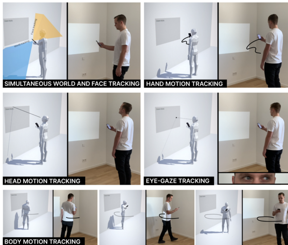
Figure 4.6: In summary, Simo implements simultaneous use of the front and back camera of the smartphone for tracking of the absolute world-space pose of the user's device (hand), body, head, and eyes (gaze). Combined with touch inputs, this potentially enables, after a simple app download, any smartphone user to perform powerful multimodal spatial interactions for distant displays.
