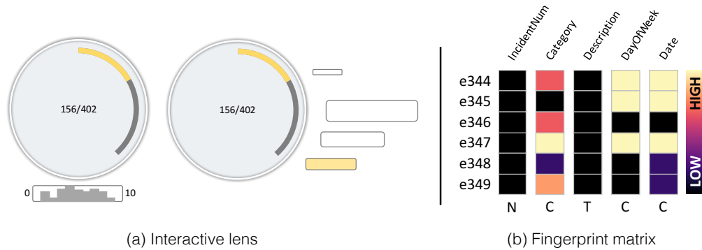
Figure 3.5: (a) The interactive lens consists of three additional parts: a textual indication of selected points, a radial histogram, and the visualization of the values included in the selection. Left: visualization of the quantified content by a histogram. Right: visualization of the content by labels. (b) Excerpt from the fingerprint matrix for five attributes and six entries. The value of each attribute is binned based on the quantification. The size of the bin is then mapped to the color. This example shows that all IncidentNum are unique, because the color of all rows refers to the lowest possible value. In contrast, the attribute DayOfWeek indicates that the data entries happen on at least four different days: three rows are mapped to black (unique) and three have a very high binning value, meaning that these entries possibly share the same day.
