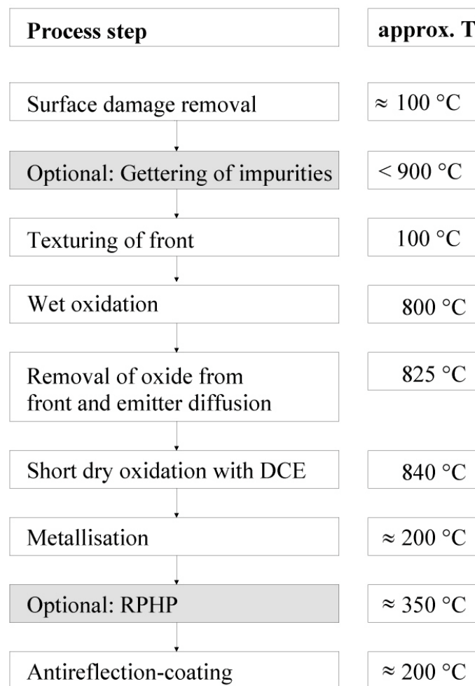
Fig. 6.12: Process sequence for high-efficiency multicrystalline silicon solar cells and approximate process temperatures. The getting in the beginning and the hydrogen passivation at the end (RPHP) are optional and not necessary for very clean material.
