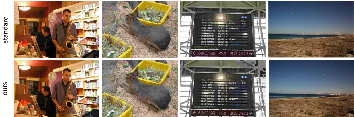
Figure 2.5: Standard JPEG vs. our variable coding strategy at the same bitrate. Some of the best parameter settings for the images in our collection with respect to DMOS. The salient parts of the image are considerably better quality than the less important and less noticeable background details. Refer to Table 2.10 for the parameters and study results for each image.
