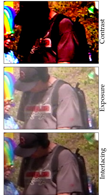
Figure 3.2: Upscaled examples of video quality defects. Courtesy to the AGH Video Quality of Experience Team for the visualizations. https://qoe.agh.edu.pl/indicators/
