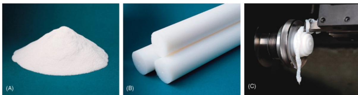
Figure 1.12. Typical processing steps to manufacture UHMWPE components. 195 Left: UHMWPE resin powder. Center: semi-finished rods that have been consolidated from the resin powder. Right: machining of the UHMWPE rods on a lathe. Reprinted with permission from Elsevier (Kurtz, S. M. in UHMWPE Biomaterials Handbook 2016 , Copyright 2016).
