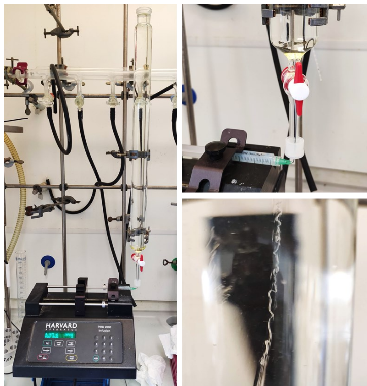
Figure 7.15. Setup to extrude dispersion and form fibers in upward direction (in ethylene glycol at room temperature).
