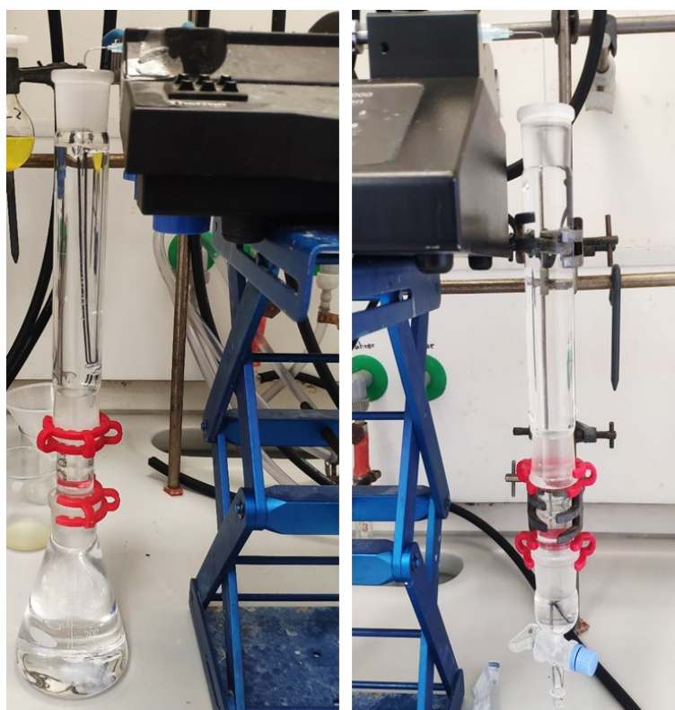
Figure 7.14. Setup modifications to gently collect the spun fibers. Left: Flask connected to a column and filled with coagulation agent to allow for post-processing of fibers in solution. Right: Column with tap connected to the bottom outlet. The coagulation agent could be gently released to prevent breakages of fibers in their sensitive wet state.
