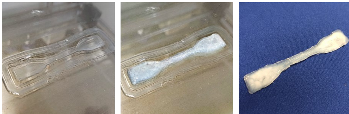
Figure 7.11. 3D UHMWPE nanocrystal paste printing following a layer-by-layer approach. The first layer was printed directly on the printer's glass bed and subsequently heated to 90 °C to evaporate water ( left ). Several layers were added (without skirt) and the water removed after every layer (center, 5 layers). The glass bed including the specimen was heated in a dry cabinet to 115 °C for several hours to remove traces of water, repair structure breakages and detach the specimen ( right ).
