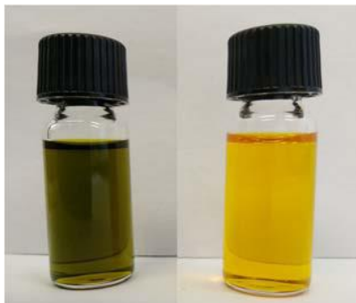
Figure 5-6: Appearance of algae oils extracted according to Folch (left) and with scCO 2 (right), respectively, diluted in CH 2 Cl 2 , showing the differences in pigment extraction. The Folch extraction also extracts chlorophylls, while scCO 2 extracts carotenoids selectively.
