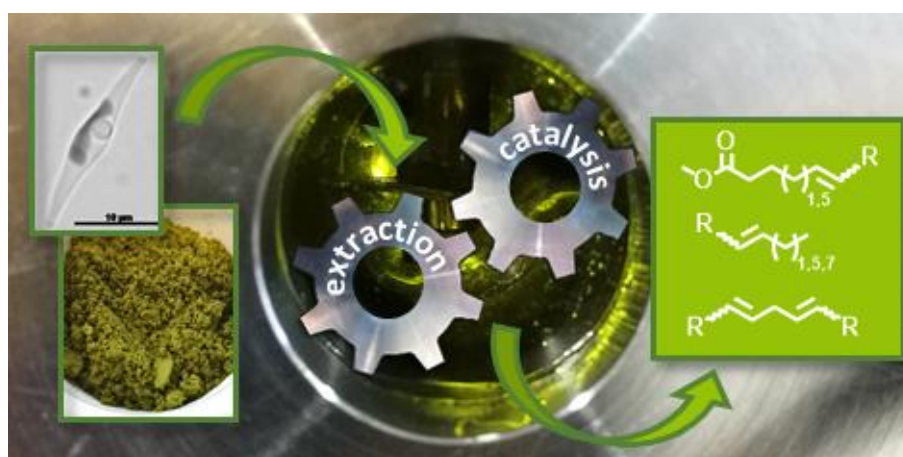
Figure 5-17: Schematic representation of the integrated extraction and catalytic upgrading of algae oil to higher value chemical building blocks.
