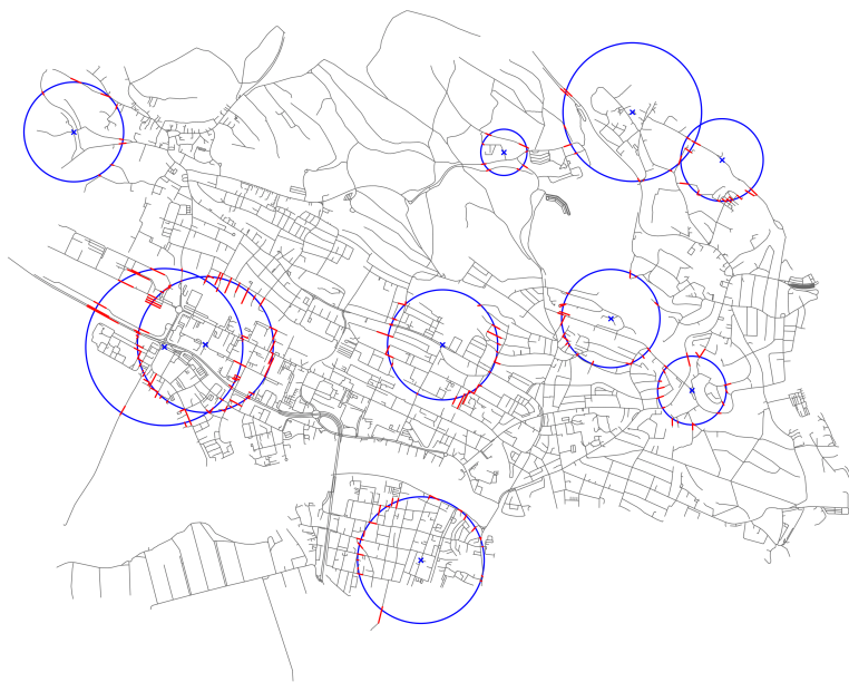
■ Figure 2 Exemplary circle-segment intersection queries with different radii on a connected road network. Query circles are blue and the respective intersecting segments are highlighted in red.
