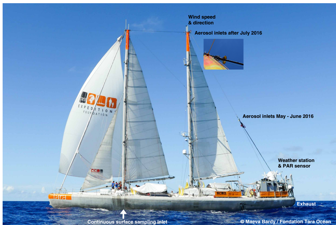
Fig. 2. R/V Tara instrument setup for the Tara Pacific Expedition . The inlet for aerosol sampling was installed along the backstay. For the first Atlantic crossing the inlet was installed halfway up the backstay. The main water entrance is located in the hull 1.5 m under the waterline; depending on ocean conditions the water will be sampled between 0.5 and 3 m under the sea surface. A detailed description of the surface water measurements can be read in Gorsky et al. (2019), and the coral reef measurements in Planes et al. (2019).
