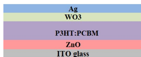
Figure 4.1.: Architecture of flat organic solar cells.
