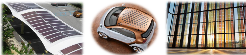
Figure 1.2.: Conceptual applications for organic solar cells (OSCs). Left: Konarka roof-top OSCs for parking canopies.[6] Middle: roof-top OSCs for the concept car "Smart Forvision".[7] Right: semi-transparent OSCs for SwissTech Convention Center. This picture was made by Solaronix (Photographer: David Martineau).[8]
