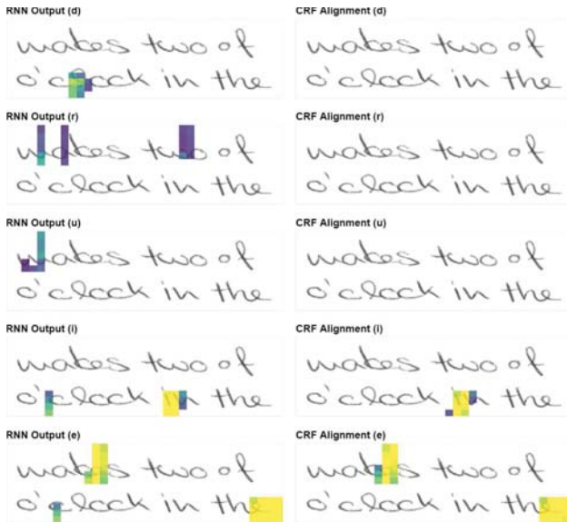
Figure 7: Heat maps of top-5 characters when using Ghosting as the sort criterion. Ghosting sort criterion shows “false-positive” characters first, which occurs e.g. at truth data errors. Left column shows the predicted probabilities, right column the alignment probabilities.
