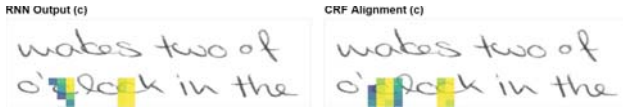
Figure 1: Example of our proposed visualization technique to a single character of a data sample. This visualization allows to quickly compare the expected and actual model prediction in relation to the neural network input. Please note that the heat map pixel size is different from the image pixel size because of spatial subsampling applied in the model.
