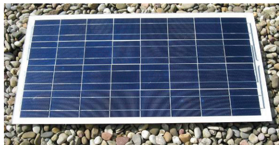
Figure 4: Demonstrator module based on 32 EpiWE cells (see text) made on monocrystalline Cz silicon wafers. Aperture area efficiency: 13.0%. Photo courtesy Fraunhofer ISE.
