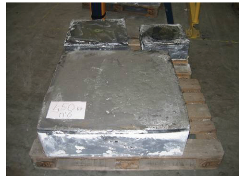
Figure 3: Ingots of 600 kg mass from Deutsche Solar (left) and 450 kg from Photowatt (right). Photos courtesy Deutsche Solar and Photowatt.
